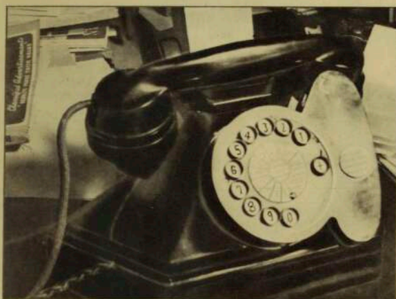
The Device Is Not Cumbersome, as this picture illustrates, and is simply manipulated. Notice that the new dial has an extra "X." This "X" is dialled before each number, which is then recorded automatically on a white paper tape.
